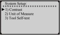
2) From the Vehicle Diagnosis menu: Use the UP/DOWN Scroll Buttons to select System Setup and then press the Y button. Follow the instructions to make adjustments and settings as described in the following setup options.
