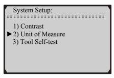
2) From the **Unit of Measure** menu, use the **UP/DOWN** scroll buttons to select the desired unit of measurement.
