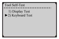
2) Press any key to start test. When you press a key, the key name should be observed on the display. If the name does not show up, then the key is not functioning properly.
