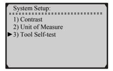
2) Select **Display Test** from the **Tool Self-Test** menu and press the **Y** button.
