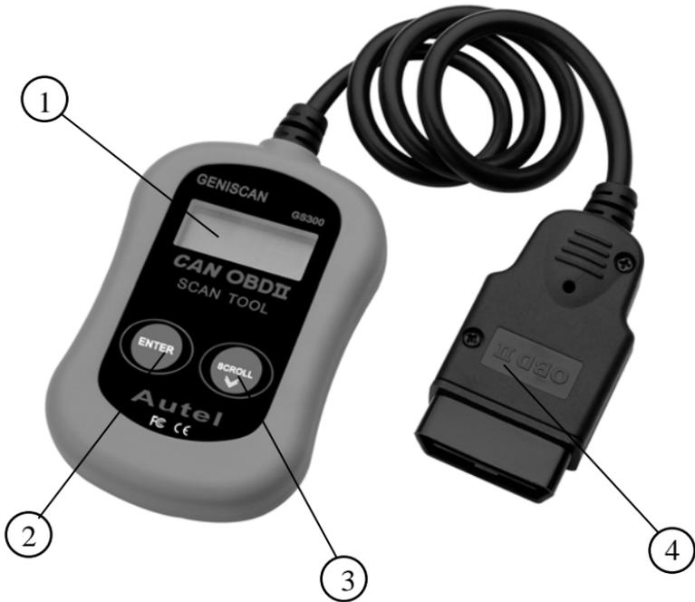
1. **LCD DISPLAY**--Indicates test results. It is a backlit 2-line display with 8 characters on each line.
